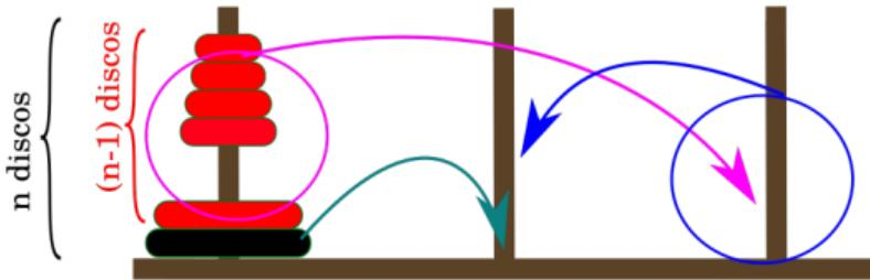
$$\begin{aligned} T(n) &= 2 T(n-1) + 1 \\ T(1) &= 1 \end{aligned}$$
